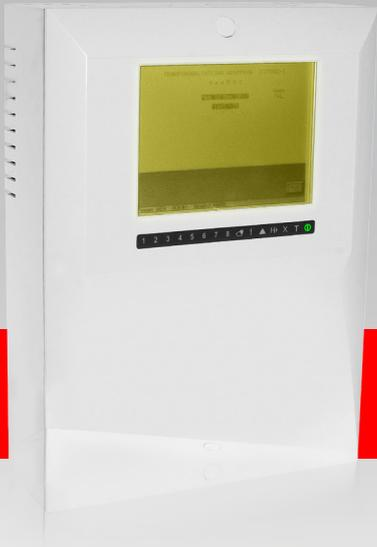
The IFS7002R repeater panel allows vital information from the IFS7000 system to be communicated through points around the building, remote from the fire alarm control panels. Distributed at strategic points in a facility - such as nurse stations, floor landings, control rooms - valuable time can be saved when identifying the location of a fire and evacuating the building.
