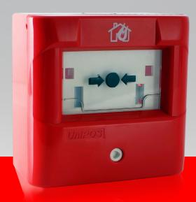
The Manual Call Point FD3050 is designed to release a signal for a fire condition to the Fire Control Panel upon manual activation by breaking the glass on the place signed with arrows. The light indication for activating the manual call point is provided by a red LED. There is a possibility for testing by a special key.
